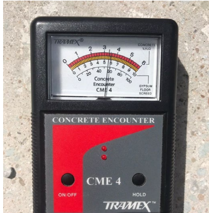
Concrete substrate moisture test - 3.4%
